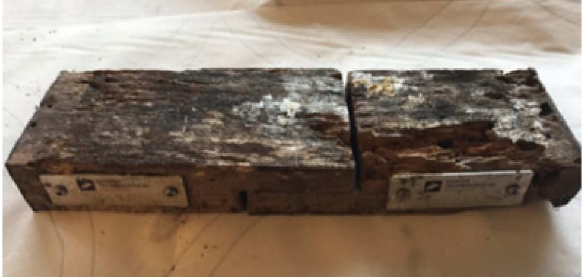
Unmodified reference sample – failed after 3 years
