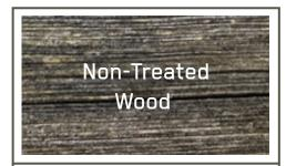
Severe signs of decay after 6 years of field testing.
