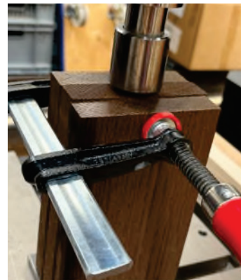
Modified test setup for longitudinal direction to prevent cracking
