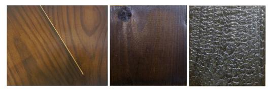
**Figure 5.** From left: Surfaces formed by compressive contact heating of pine at 260 °C, contact heating of spruce at 320 °C, gas flame charring of spruce (M. Kymäläinen).
