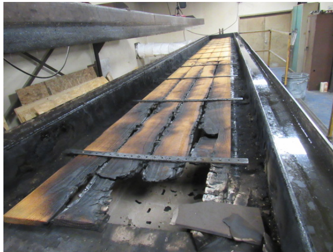
Photo No. 3 Unexposed Surface of the Test Specimen (Post-test)
